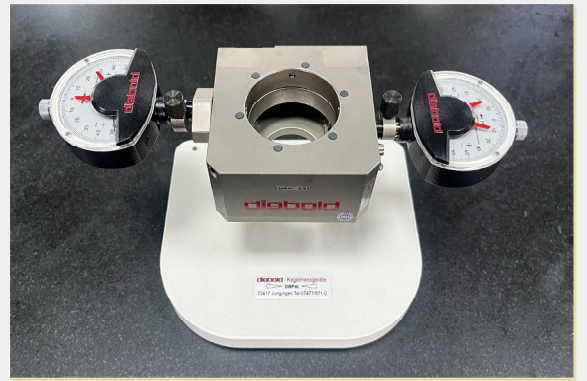
1: 10锥度检测工具图 (德国戴博刀柄检具) Picture of 1:10 taper inspection tool (German Daibo collet chuck inspection tool)
