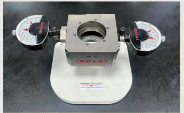
1: 10锥度检测工具图 (德国戴博刀柄检具) Picture of :1:10 taper inspection tool (German Daibo collet chuck inspection tool)
