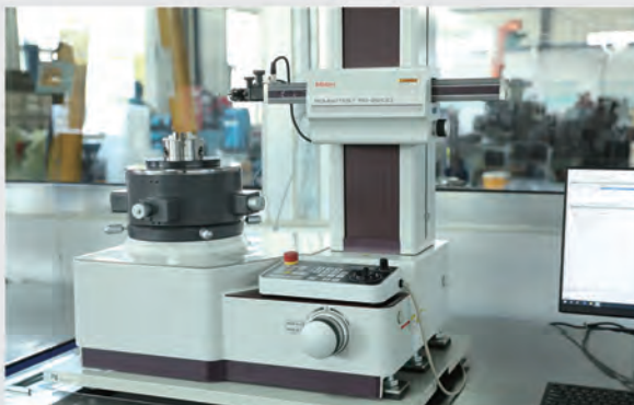
日本三丰真圆度仪 Japanese Mitutoyo Round Test Machine
