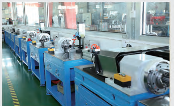
电主轴检测线 Electric Spindle Test Machines
