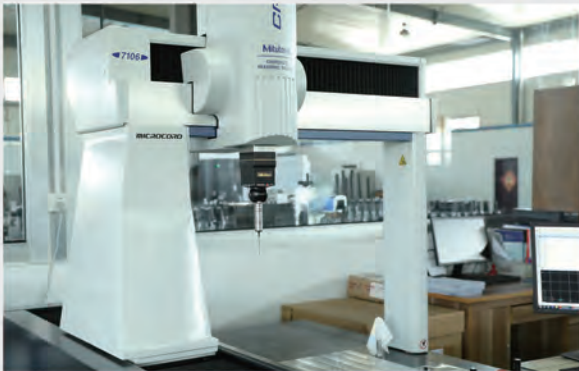
日本三丰三坐标检测仪 Mitutoyo Coordinate Measuring Machine
