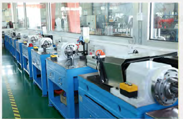
电主轴检测线 Electric Spindle Test Machines
